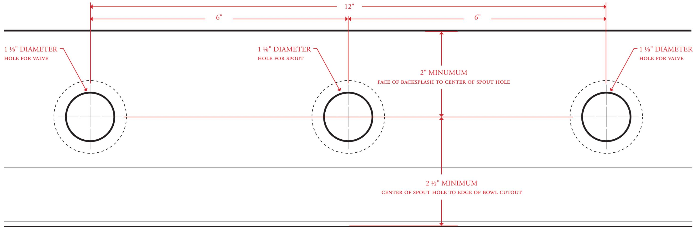
Rectangular porcelain sink with 1 1/4" undermount lip shown as example. Recommendation is for most stock basin sets; drilling for made-to-order basin sets should be confirmed individually. N° 14000 Ritz Basin Set requires 2 1/2" minimum distance from center of spout hole to edge of bowl cutout. Dashed circles indicate mounting nuts; if adjusting position ensure there is 1 3/4" clearance around drilled holes for mounting hardware. Drawing shown at scale on tabloid.
