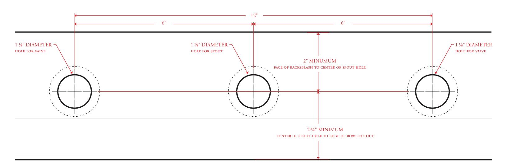
Rectangular porcelain sink with 1 ¼" undermount lip shown as example. Recommendation is for most stock basin sets; drilling for made-to-order basin sets should be confirmed individually. N° 14000 Ritz Basin Set requires 2 ½" minimum distance from center of spout hole to edge of bowl cutout. Dashed circles indicate mounting nuts; if adjusting position ensure there is 1 ¾" clearance around drilled holes for mounting hardware. Drawing shown at scale on tabloid.
