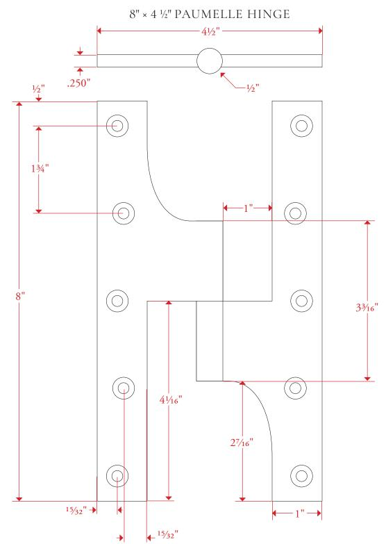
All measurements are in inches unless otherwise noted. Drawing shown at ¾ scale. Please do not scale drawing. Template is for reference only, not mortising purposes. All field cutting and fitting should be done with physical hardware. Right hand hinge shown; please specify hand when ordering. All barrels are ½" diameter however diameter will change depending
