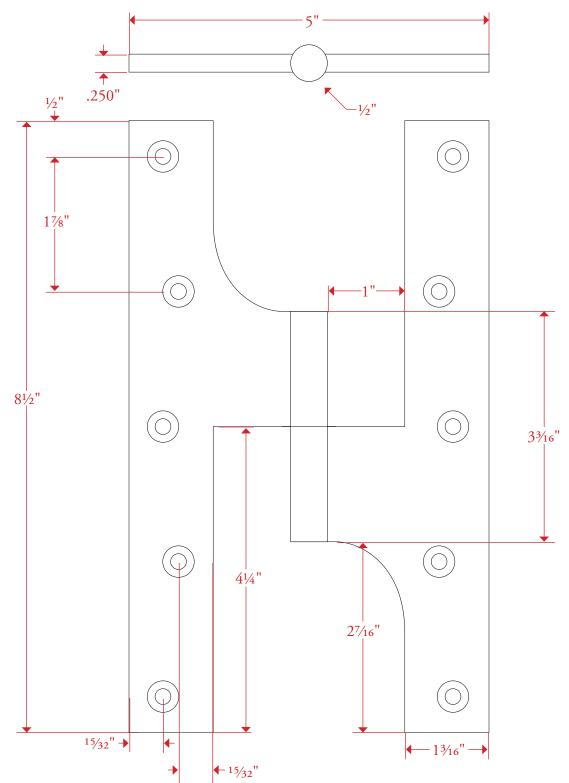
All measurements are in inches unless otherwise noted. Drawing shown at ¾ scale. Please do not scale drawing. Template is for reference only, not mortising purposes. All field cutting and fitting should be done with physical hardware. Right hand hinge shown; please specify hand when ordering. All barrels are ½" diameter however diameter will change depending
