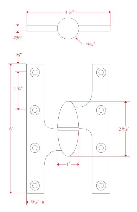
All measurements are in inches unless otherwise noted. Drawing shown at ¾ scale. Please do not scale drawing. Template is for reference only, not mortising purposes. All field cutting and fitting should be done with physical hardware. Drawing is approximate for showing overall dimensions.
