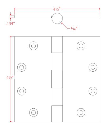
All measurements are in inches unless otherwise noted. Drawing shown at ¾ scale. Please do not scale drawing. Template is for reference only, not mortising purposes. All field cutting and fitting should be done with physical hardware.
