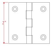
All measurements are in inches unless otherwise noted. Drawing shown at ¾ to scale. Please do not scale drawing. Template is for reference only, not mortising purposes. All field cutting and fitting should be done with physical hardware.
