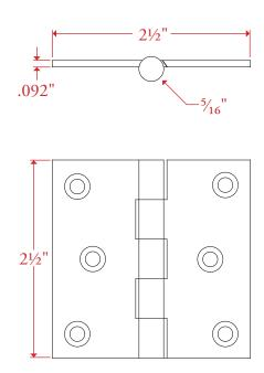
All measurements are in inches unless otherwise noted. Drawing shown at ¾ to scale. Please do not scale drawing. Template is for reference only, not mortising purposes. All field cutting and fitting should be done with physical hardware.
