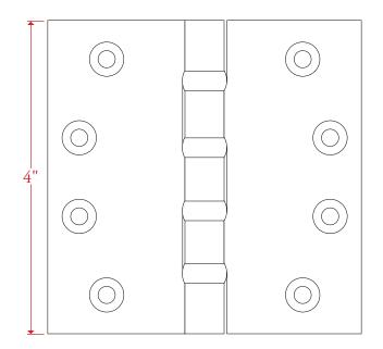
All measurements are in inches unless otherwise noted. Drawing shown at ¾ scale. Please do not scale drawing. Template is for reference only, not mortising purposes. All field cutting and fitting should be done with physical hardware.
