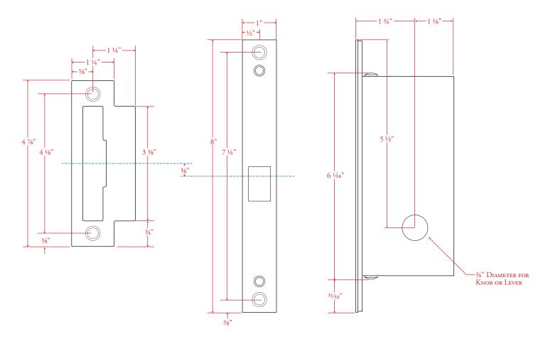
Drawing shown at ½ scale. Please do not scale drawing. Template is for reference only, not mortising purposes. All field cutting and fitting should be done with physical hardware.
