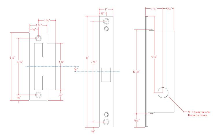
Drawing shown at ½ scale. Please do not scale drawing. Template is for reference only, not mortising purposes. All field cutting and fitting should be done with physical hardware. Please note when mounting hardware, face plate and strike use #12-24 flat head screws.
