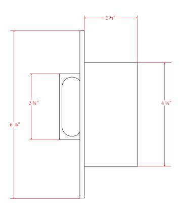
Drawing shown at ½ scale. Please do not scale drawing. Template is for reference only, not mortising purposes. All field cutting and fitting should be done with physical hardware. Please note when mounting hardware, face plate uses #7 flat head screws.
