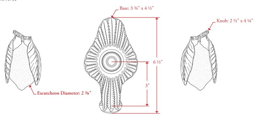
All measurements are in inches unless otherwise noted. Drawing shown at ½ scale. Please do not scale drawing. Template is for reference only, not mortising purposes. All field cutting and fitting should be done with physical hardware. Drilling Instructions: Hole sizes to be 1½" minimum for installation of valves and spout.
