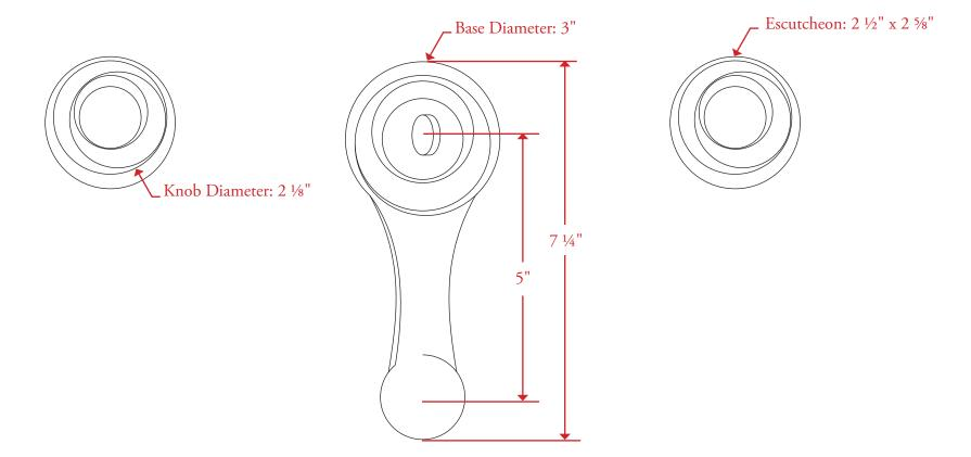
All measurements are in inches unless otherwise noted. Drawing shown at ½ scale. Please do not scale drawing. Template is for reference only, not mortising purposes. All field cutting and fitting should be done with physical hardware. All matching bathroom accessories are available. Drilling Instructions: Hole sizes to be 1 %" minimum for installation of valves and spout.
