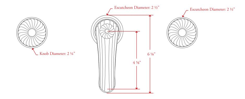
All measurements are in inches unless otherwise noted. Drawing shown at ½ scale. Please do not scale drawing. Template is for reference only, not mortising purposes. All field cutting and fitting should be done with physical hardware. All matching bathroom accessories are available. Drilling Instructions: Hole sizes to be 1 ½" minimum for installation of valves and spout.
