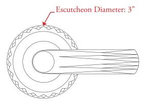
All measurements are in inches unless otherwise noted. Drawing shown at ½ scale. Please do not scale drawing. Template is for reference only, not mortising purposes.
