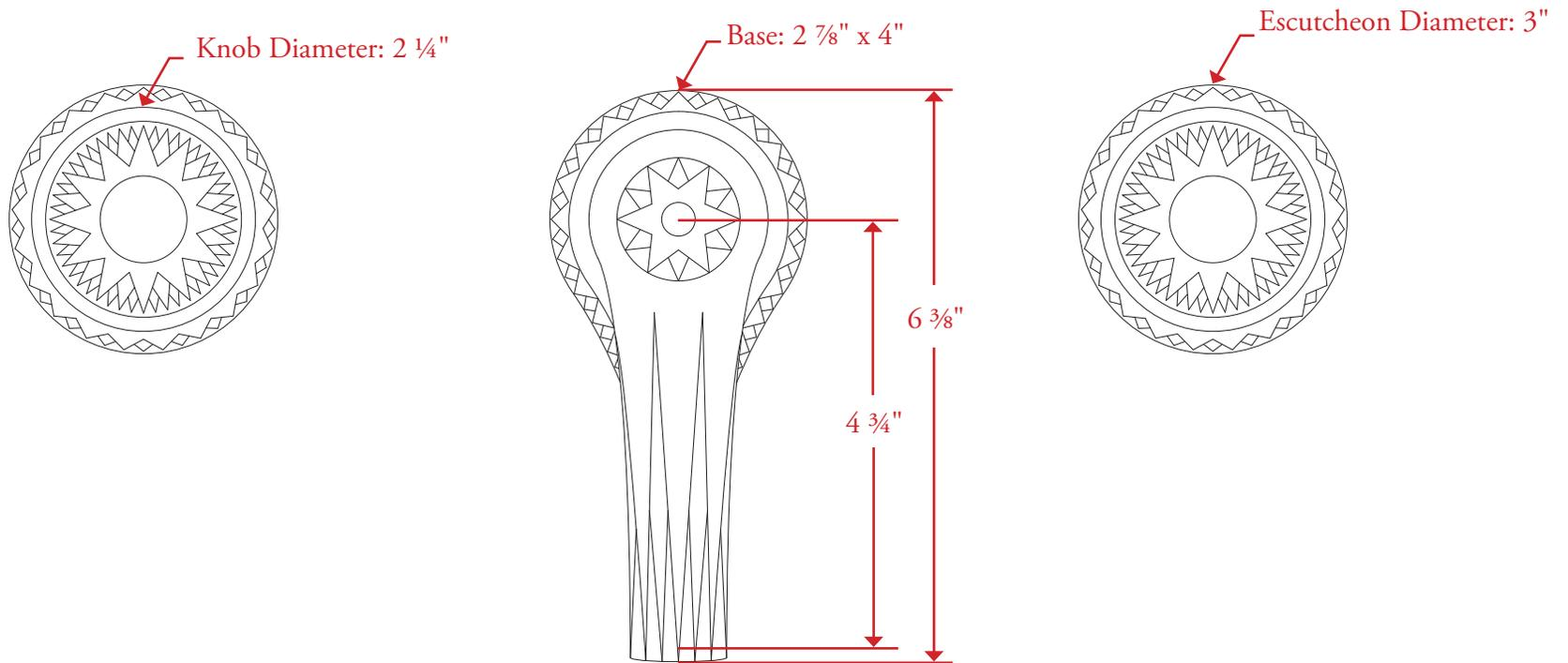
All measurements are in inches unless otherwise noted. Drawing shown at 1/2 scale. Please do not scale drawing. Template is for reference only, not mortising purposes.
