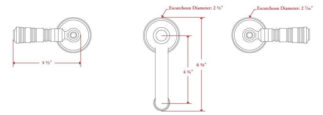
All measurements are in inches unless otherwise noted. Drawing shown at ½ scale. Please do not scale drawing. Template is for reference only, not mortising purposes. All field cutting and fitting should be done with physical hardware. All matching bathroom accessories are available. Drilling Instructions: Hole sizes to be 1 1%" minimum for installation of valves and spout.
