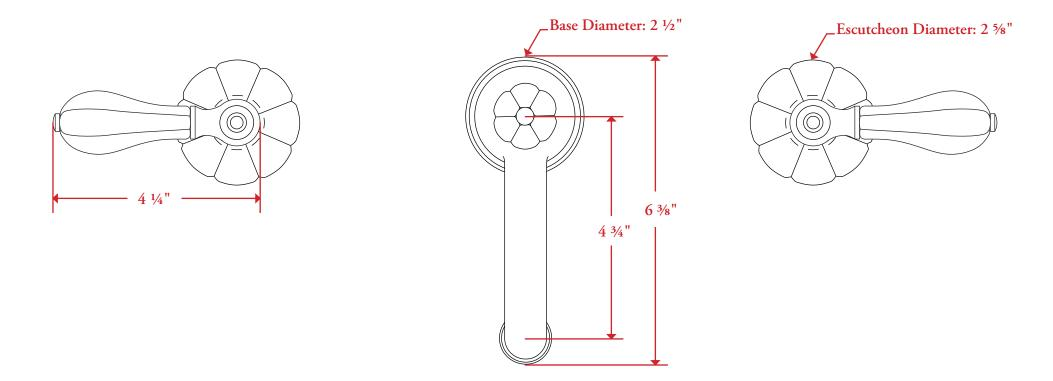
All measurements are in inches unless otherwise noted. Drawing shown at ½ scale. Please do not scale drawing. Template is for reference only, not mortising purposes. All field cutting and fitting should be done with physical hardware. All matching bathroom accessories are available. Drilling Instructions: Hole sizes to be 1 ½" minimum for installation of valves and spout.
