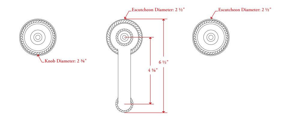
All measurements are in inches unless otherwise noted. Drawing shown at ½ scale. Please do not scale drawing. Template is for reference only, not mortising purposes. All field cutting and fitting should be done with physical hardware. All matching bathroom accessories are available. Drilling Instructions: Hole sizes to be 1 ½" minimum for installation of valves and spout.
