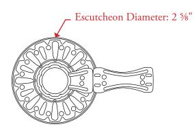
All measurements are in inches unless otherwise noted. Drawing shown at ½ scale. Please do not scale drawing. Template is for reference only, not mortising purposes. All field cutting and fitting should be done with physical hardware. All matching bathroom accessories are available. Drilling Instructions: Hole sizes to be 1 ½" minimum for installation of valves and spout.
