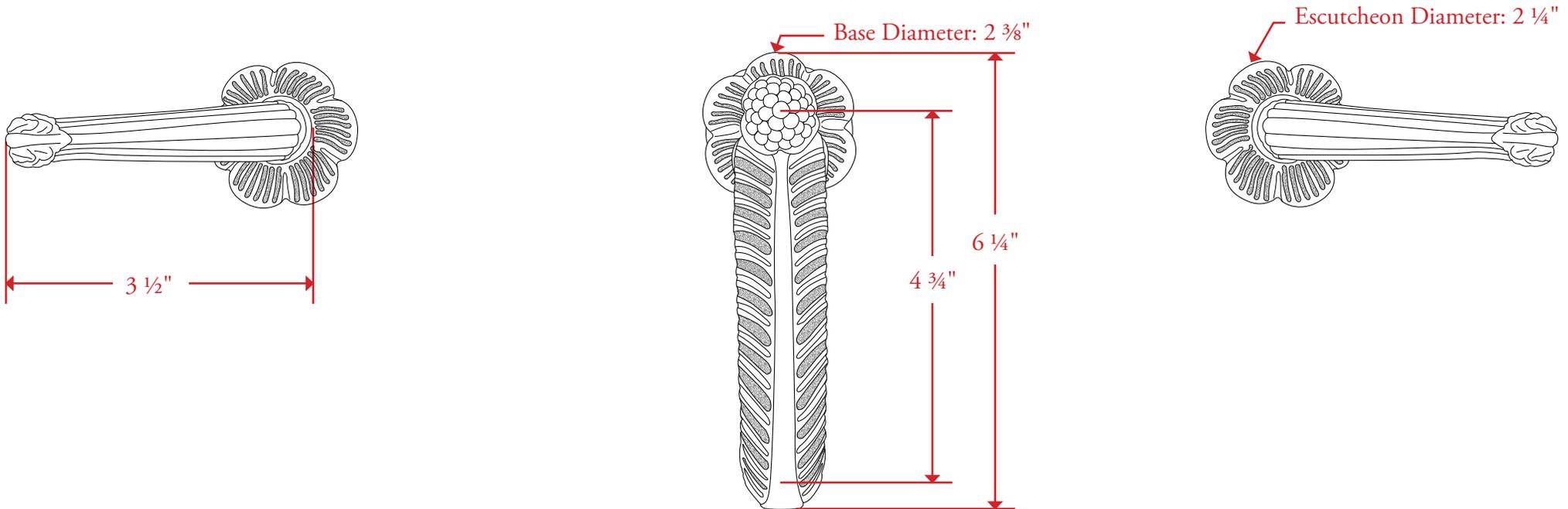
All measurements are in inches unless otherwise noted. Drawing shown at  $\frac{1}{2}$  scale. Please do not scale drawing. Template is for reference only, not mortising purposes. All field cutting and fitting should be done with physical hardware. The Lotus Basin Set is made to order and is available as a complete collection. All matching bathroom accessories are available. Some spout designs require additional mounting space. Please verify clearance at basin or tub.
