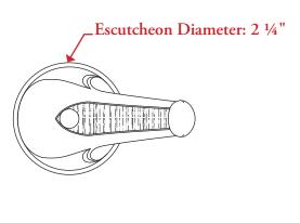
All measurements are in inches unless otherwise noted. Drawing shown at ½ scale. Please do not scale drawing. Template is for reference only, not mortising purposes. All field cutting and fitting should be done with physical hardware. All matching bathroom accessories are available. Drilling Instructions: Hole sizes to be 1 1%" minimum for installation of valves and spout.
