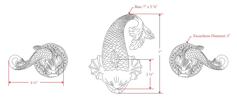
All measurements are in inches unless otherwise noted. Drawing shown at ½ scale. Please do not scale drawing. Template is for reference only, not mortising purposes.
