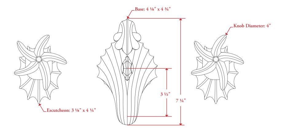
All measurements are in inches unless otherwise noted. Drawing shown at ½ scale. Please do not scale drawing. Template is for reference only, not mortising purposes. All field cutting and fitting should be done with physical hardware. All matching bathroom accessories are available. Drilling Instructions: Hole sizes to be 1 ½" minimum for installation of valves and spout.
