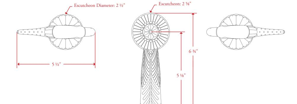
All measurements are in inches unless otherwise noted. Drawing shown at ½ scale. Please do not scale drawing. Template is for reference only, not mortising purposes. All field cutting and fitting should be done with physical hardware. All matching bathroom accessories are available. Some spout designs require additional mounting space. Please verify clearance at basin or tub.
