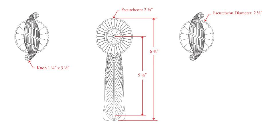
All measurements are in inches unless otherwise noted. Drawing shown at ½ scale. Please do not scale drawing. Template is for reference only, not mortising purposes. All field cutting and fitting should be done with physical hardware. All matching bathroom accessories are available. Some spout designs require additional mounting space. Please verify clearance at basin or tub.
