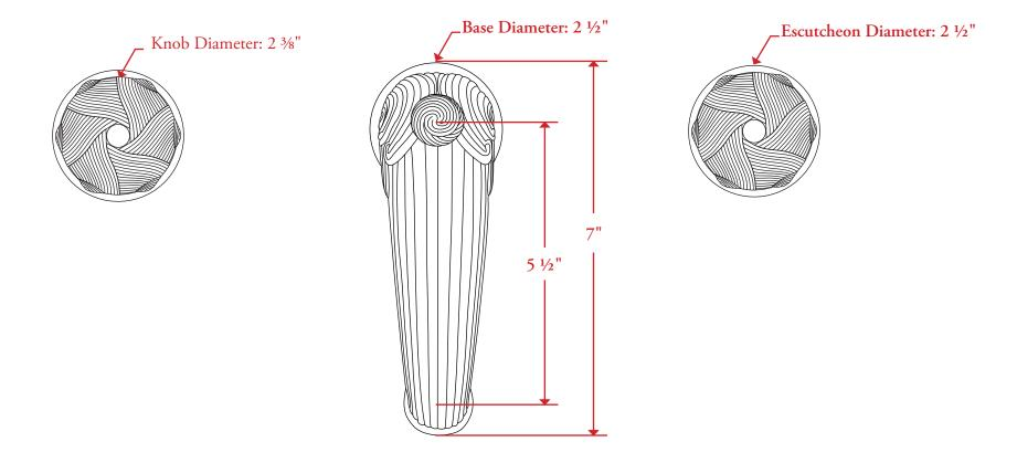
All measurements are in inches unless otherwise noted. Drawing shown at ½ scale. Please do not scale drawing. Template is for reference only, not mortising purposes. All field cutting and fitting should be done with physical hardware. All matching bathroom accessories are available. Drilling Instructions: Hole sizes to be 1 ½" minimum for installation of valves and spout.
