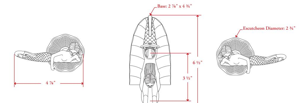
All measurements are in inches unless otherwise noted. Drawing shown at ½ scale. Please do not scale drawing. Template is for reference only, not mortising purposes. All field cutting and fitting should be done with physical hardware. All matching bathroom accessories are available. Drilling Instructions: Hole sizes to be 1 1%" minimum for installation of valves and spout.
